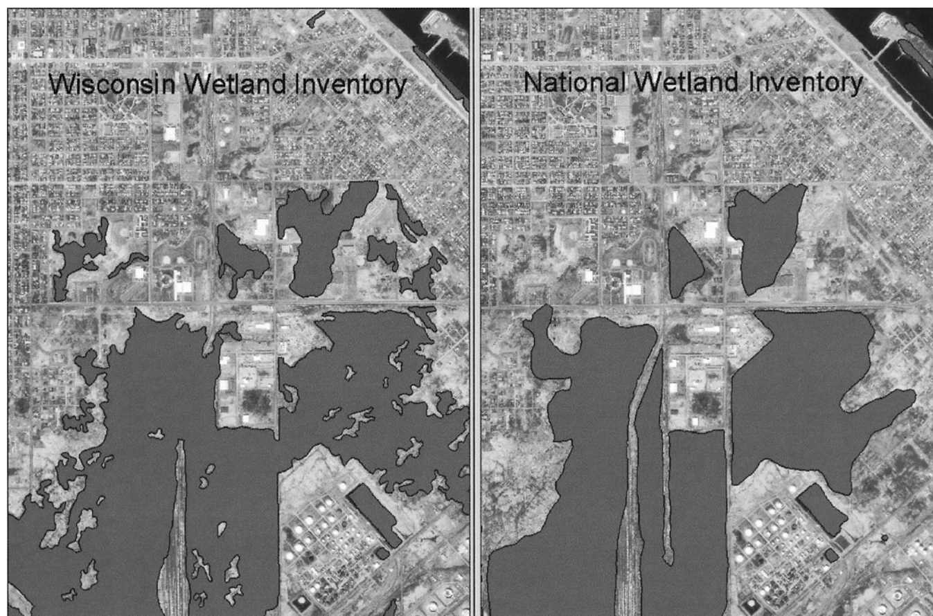
Figure 4. Comparison of boundary complexity between the two inventories in a portion of the Superior study area (sections 23–26, T49N, R14W). Grey shading masks all Palustrine wetlands (wet forests, shrub swamps, wet meadows, and excavated ponds) mapped by the Wisconsin Wetlands Inventory (left side) and the National Wetlands Inventory (right side). The U.S.G.S. digital orthophoto backdrop is identical on both sides, and was not an information source for either inventory.
